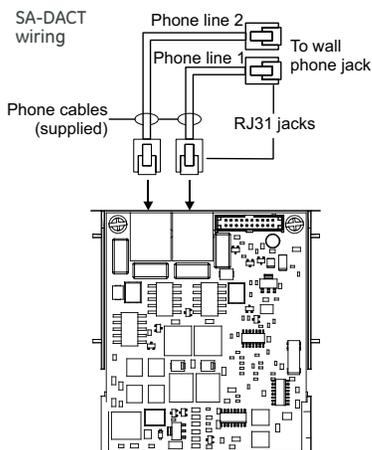
The dialer phone lines connect to connectors on the dialer's main circuit board. Phone line 1 connects to connector J4 and phone line 2 connects to connector J1.
