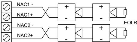
Marking indicates output signal polarity when the circuit is active. Polarity reverses when the circuit is not active. Wire notification appliances accordingly. Notification appliance polarity shown in active state.
